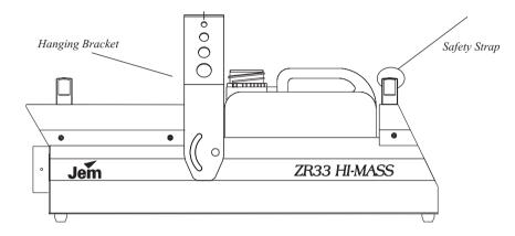
The ZR33 flying kit enables the machine to be fixed to rigging and ceilings for use where the ZR33 is best situated in a flying position. The kit is supplied as standard with the option of a drip pad for catching unwanted drips that can occur when smoke machines are angled down.
