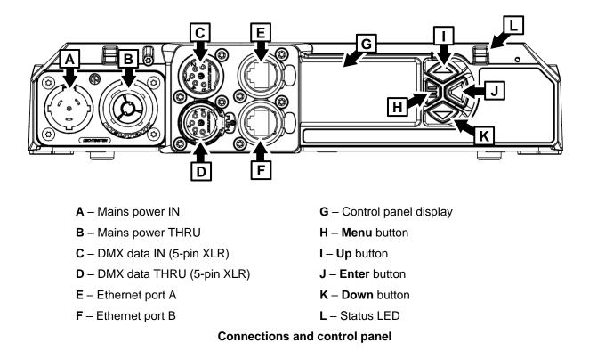
When the MAC One is powered on, it first boots and resets, then it displays its DMX address (or its fixture ID number, if one has been set) and any status messages (see 'Service and diagnostic messages' on page 35) in the display **G**. The display can be set to automatically rotate to match standing or hanging fixture orientation in the PERSONALITY  $\rightarrow$  DISPLAY menu or the Shortcuts menu (see 'Shortcuts menu' on page 11).
